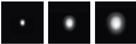
S = spot (8°-15°) F = flood (15°-30°) WF = wide flood (30°-45°)
