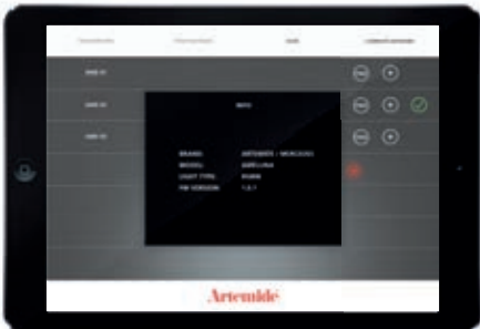
Find physical lamp phase The lamp will signal itself by blinking
