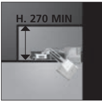
Special application without Carter against the wall.
